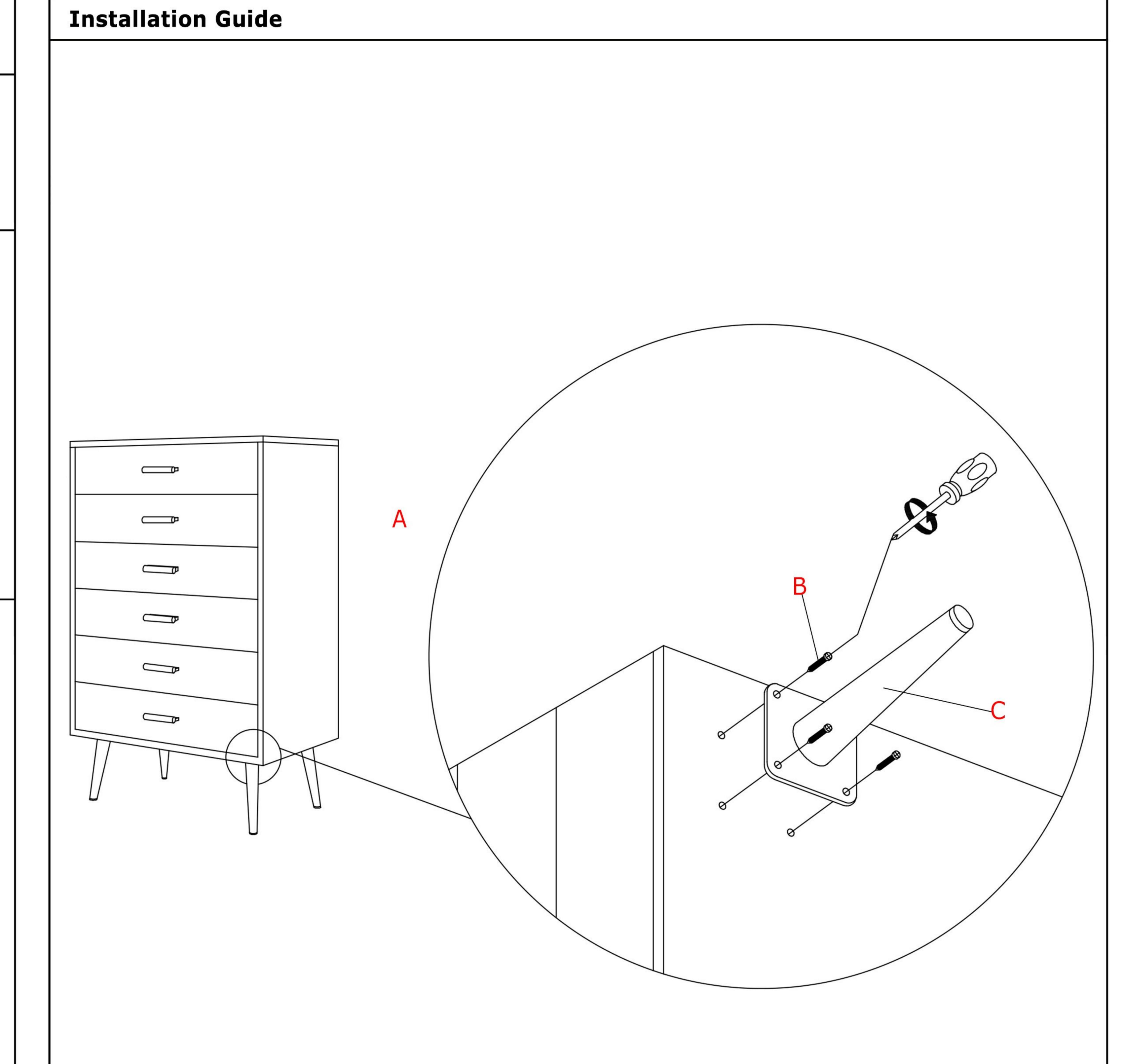
1. Fix the legs (C) to the corresponding holes on the bottom of the cabinet body (A) with screws (B) and a screw driver as shown in the picture.
